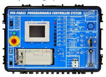
directly related to industry needs, including using a six-step sequence to troubleshoot a PLC system, troubleshooting a PLC routine that performs on/off control using an analog input, and testing a PLC-controlled Pulse-Width Modulation (PWM) output device.
